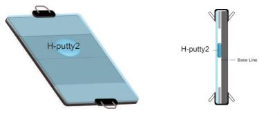
Material no dropped or changed after high temperature aging testing
